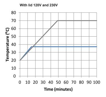
Heat up time from 20°C. Bath shaking with linear motion at 110rpm.
