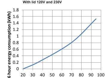
Consumption is measured over a 6 hour period when the bath is controlling at set temperature and shaking at 110rpm. All figures are for guidance only. Consumption figures may vary due to factors such as ambient temperature, vessel loading, shaking speed & ventilation.
